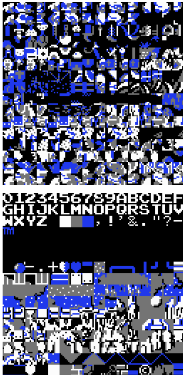
Figure 2: Pattern tables for the Zelda overworld. In Zelda, the top tiles are used for sprites, and the bottom are used for the background graphics. All tiles are 8x8 and use 4 color values (color 0 is transparent). These color values index into 4 sprite palettes and 4 background palettes, with some limitations.
